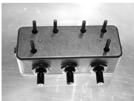
Fig. 4. Die cast aluminum enclosure with brass sticks as interface connectors. On the front are potentiometers to modify internal parameters of the electronic circuit.
