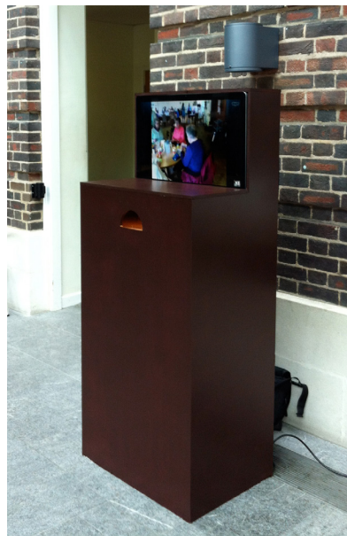
Fig. 3. The Teletalker during field research in the quadrangle of Middlesex University. This photo shows the hole in the body of the Teletalker at the height of 105cm and the light shining out of the hole. The user needs to place their hand into the hole, covering the light-sensitive resistor, in order to activate the volume.
