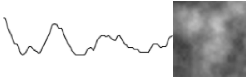
Fig 2b. The Perlin-Noise function: function graph and 2D pattern of grey values.
