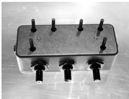
Fig. 4. Die cast aluminum enclosure with brass sticks as interface connectors. On the front are potentiometers to modify internal parameters of the electronic circuit.
